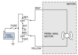
\*Note: Red for Electrak 1 White for 12VDC Electrak 1 with Feedback Black for 24VDC Electrak 1 with Feedback
