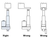
The actuator mounting brackets must be able to withstand the torque which is developed when the unit extends or retracts. Restraining torque required varies with the model being used.
