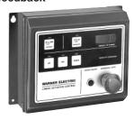
An advanced control unit for the new Electrak 205 actuator with a digital LCD meter to display the feedback position and a 4-20 mA output signal to operate a remote meter or provide an input to a programmable controller. Same membrane function switches as the MCS-2035.
