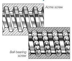
Electrak 1, 2, 050 and 150 models feature acme screws which will not backdrive when the power is off. Electrak 5, 10, 100 and 205 series actuators are equipped with highly efficient and accurate Warner Linear ball bearing screws. A load holding brake keeps the load in position when power is off.
